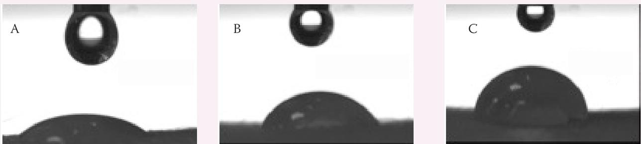
Figure 2: Comparison of the wetting behaviour (spreading of a sessile drop on human skin) of octenilin (A), Prontosan (B) and Ringer solution (C).
