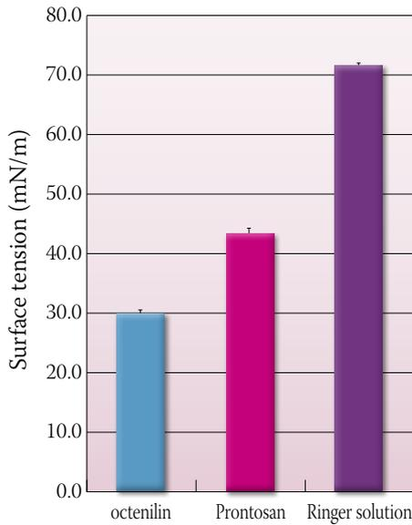
Figure 1: Comparison of the surface tension [mN/m] of octenilin, Prontosan and Ringer solution. Bars indicate standard deviations.
